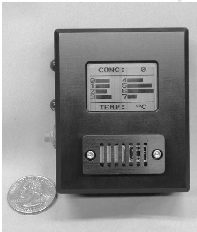
Fig. 1. Seacoast Science's SC100 Badge-Size Chemical Warfare Agent detector prototype. Dimensions: 3.3 in. × 2.7 in. × 1 in.; weight: ~8 ounces (220 g) with battery.
