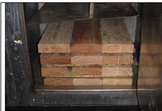
Figure 10. 23 board feet of wet southern pine loaded into the pilot-scale kiln.
