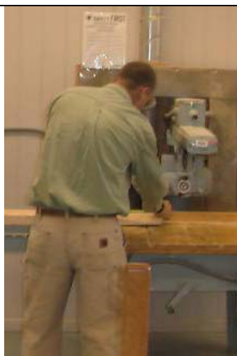
Figure 6. Wood is cut into twelve 2 x 6 x 25 inch boards.
