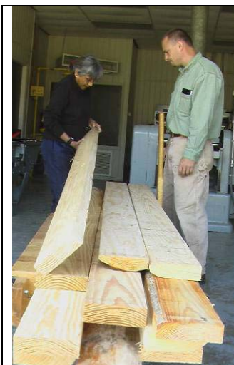
Figure 5. Sita Warren and Ruben Shmulsky grade wet Southern Pine boards.
